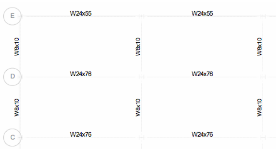
Figure 15 – Steel beam layout for P/C panels
